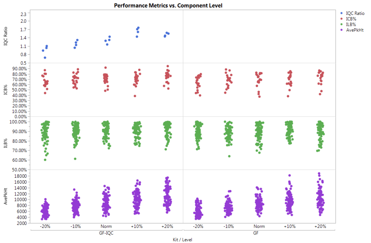
Figure 67 Primer mix amount variation for GlobalFiler™ IQC (left) and GlobalFiler™ (right) kits. Input is \pm 20\% of standard 2.5 \mu\text{L} input per 25 \mu\text{L} reaction (with standard master mix amount) with 1.0 ng of control DNA 007.
